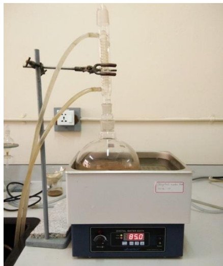
Reflux extraction at 80°C water bath
